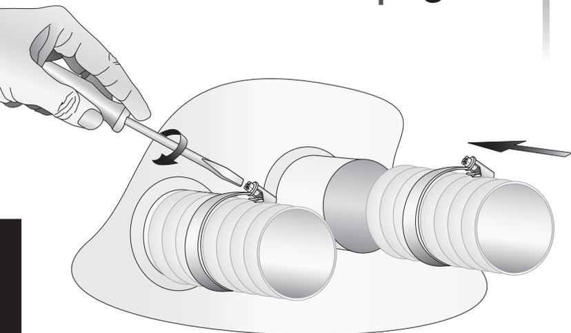
Tighten flue clamps to secure flues to the firebox.
