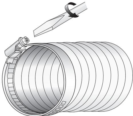
Using a flat head screwdriver, unscrew the flue clamp as necessary until it fits over the end of each of the flexi flue pipes.
